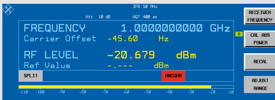
FIG 2a If absolute calibration has not been performed, the R&S®FSMR activates the red UNCORR field to warn you that the measurements may be inaccurate.
